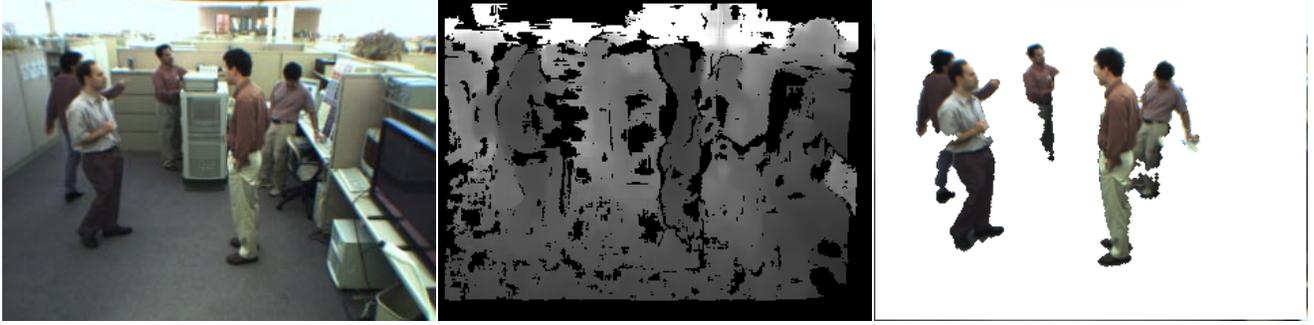
Figure 2. Example camera-view input. Left to right: (a) Color, (b) Depth (unreliable data shown in black), (c) Foreground color.
