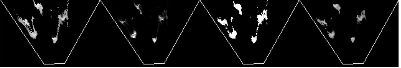
**Figure 3. Plan-view maps of the foreground of Figure 2. The stereo camera’s plan-view location is just outside the bottom of the images, and the lines indicate the camera’s field of view. Left to right: (a) Raw height map  $\mathcal{H}_{raw}$ , (b) Raw occupancy map  $\mathcal{O}_{raw}$ , (c) Bitmap showing where smoothed occupancy exceeds threshold  $\theta_{occ}$ , (d) Masked, smoothed height map  $\mathcal{H}_{masked}$ .**
