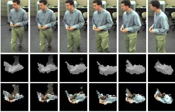
**Figure 3. Templates for tracked person over 0.9 seconds (every other frame shown). Row 1: Color input (depth not shown); Row 2: Height templates  $\mathcal{T}_H$ ; Row 3: Color templates  $\mathcal{T}_C$ . Note that head, hands, and legs are visible.**
